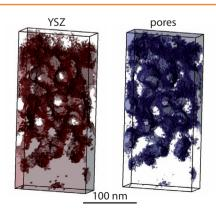
The porosity evolution of yttria-stabilized zirconia (YSZ) and gadolinium-doped ceria (CGO) thin films deposited by spray pyrolysis is presented. The pore distribution is analyzed by focused ion beam tomography. The YSZ of the reconstruction is colored in brown and the pores in blue. About 43 vol% of porosity develops during annealing at 800 °C for 20 h.
