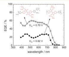
Polymer:fullerene photovoltaic devices comprising two isoindigo containing polymers show large differences in opencircuit voltage ( $V_{\rm oc}$ ) and external and internal quantum efficiencies. Instead of morphology, an almost vanishing energetic difference between the optical gap of the polymer and energy of the charge transfer state is responsible for the lower photocurrent produced by the high  $V_{\rm oc}$  device.
