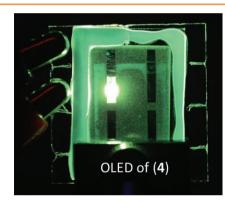
Fine-tuning the emission hue of Os(II) phosphors from saturated red to green is achieved using benzothiazolyl or benzimidazolyl chromophores plus a chelating diphosphine, from which the highly efficient PhOLEDs are fabricated using a solution process.
