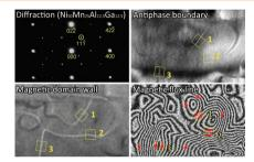
Peculiar magnetic domain walls produced in a Heusler alloy are studied using electron holography. The observations reveal unexpectedly narrow magnetic domain walls, the width of which shows perfect agreement with that of the antiphase boundaries (e.g., only 3 nm). This method provides beneficial information for obtaining a deeper understanding of the magnetic order in the vicinity of an interface.
