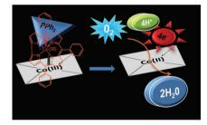
Pyrolyzed Co-corrole supported by carbon black catalyzes the oxygen reduction reaction (ORR) by a direct four-electron reduction pathway for the reduction of  $O_2$  to  $H_2O$  and exhibits high activity as the cathode catalyst of polymer electrolyte fuel cells. The pyrolysis changes the coordination structure and oxidation state of Co-corrole, leading to the increase in ORR activity.
