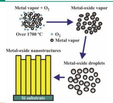
Three processes are involved in the vaporsolid (VS) growth mechanism for the synthesis of 1D metal-oxide nanostructures: i) thermal sublimation from the hot metal filament, ii) chemical vapor reaction of the sublimated heavy metal vapor with ambient oxygen gas, and iii) condensation of the heavy metal-oxide vapor into 1D nanostructures.
