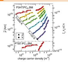
It is shown that the often reported recombination orders, which are higher than two for organic photovoltaic solar cells, cannot be explained by the charge carrier density, n, dependence of the mobility,  $\mu$ , alone, as the Langevin recombination prefactor k exhibits a different n dependence than  $\mu$ . The discrepancy is explained by a more complex recombination process including trap states and phase separation.
